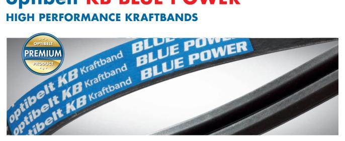
optibelt KB BLUE POWER kraftbands are made of wrapped optibelt BLUE POWER high performance wedge belts which are joined together by a highly wear-resistant top surface. This compact drive product is the preferred choice for handling extreme shock loads, large centre distances and vertical shafts.
