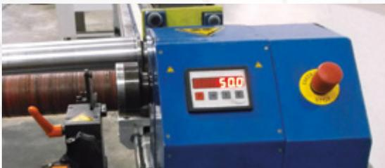
Automatic tensioning with 4 presets, large digital display, and 0.01 mm cutting accuracy.
